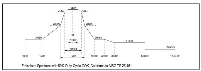
Figure 3. AISG Standard Modem Spectrum Emission Mask
