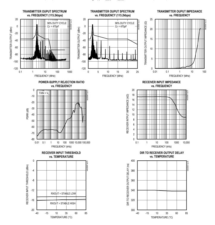
Typical Operating Characteristics ( $V_{CC}$  = 5V,  $V_L$  = 3.3V, TXOUT connected with 50Ω to RXIN, RXIN connected to 50Ω in series with 220nF to GND, R1 = 10kΩ between BIAS and RES, R2 = ∞, pullup SYNCOUT with 1kΩ to  $V_L$ ,  $T_A$  =  $T_{MIN}$  to  $T_{MAX}$ , unless otherwise specified.)
